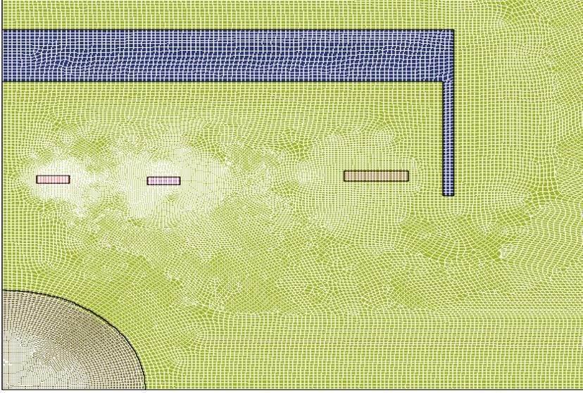
Fig 3. The finite element mesh for the model of the iron shielded superconducting magnet.
