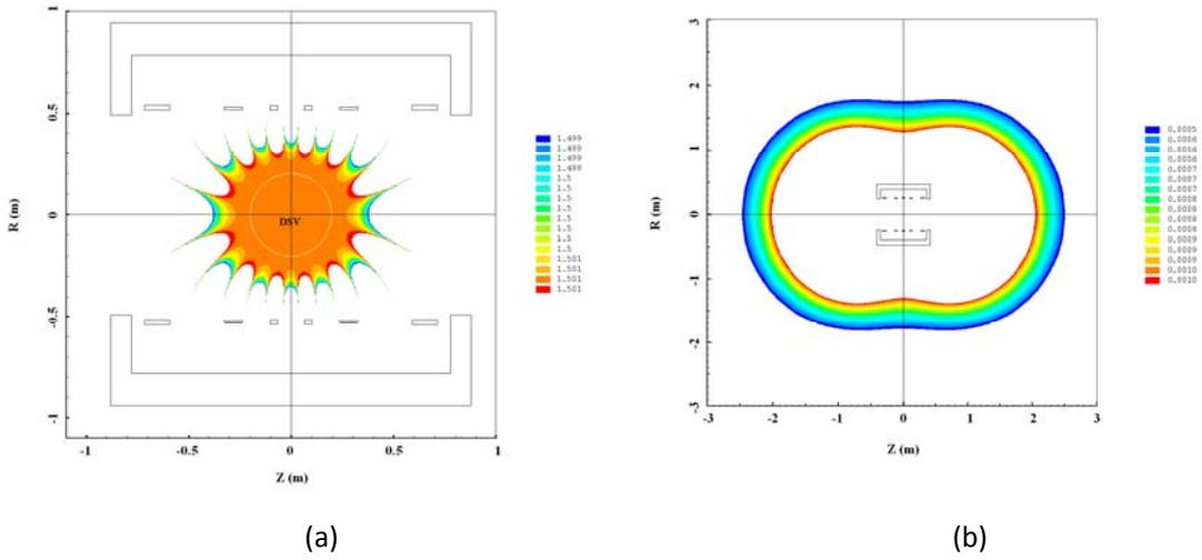
Fig 5. Computational results of the 1.5T iron shielded superconducting magnet: (a)  $B_0$  field distribution in the DSV; (b) The fringe field distribution outside the magnet.
