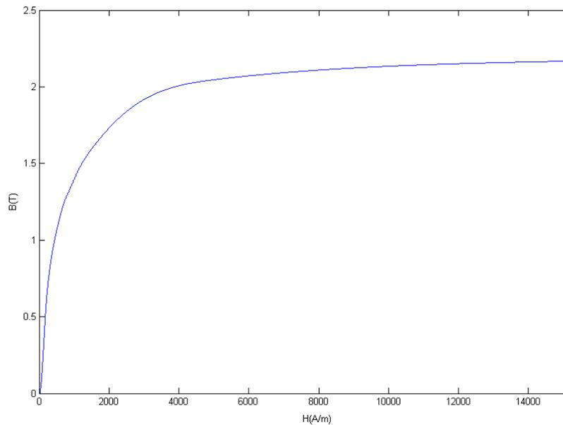
Fig. 2 The magnetization curve of the magnetic pure iron used
