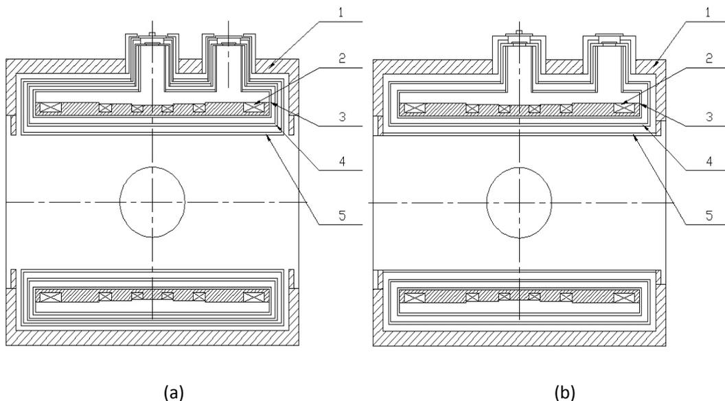
Fig 1. Schematic of iron shielded superconducting magnet: (a) A magnet with conventional iron shield. (b) The magnet adapting novel iron shield scheme. 1 - iron shield, 2 - superconducting coil, 3 - the first thermal shield enclosing the helium chamber, 4 - the second thermal shield, 5 - the third thermal shield at room temperature.
