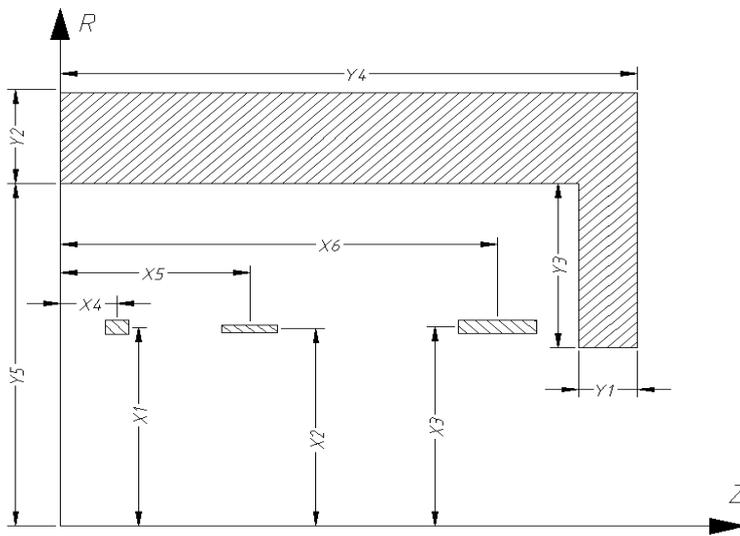
Fig 4. The geometry model of the magnet and design variables setting.
